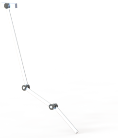
Fig. 1. CAD Model of the Triple Pendulum
